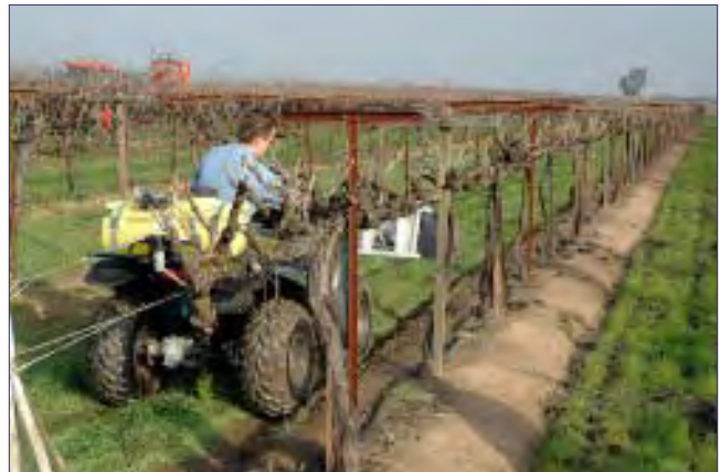
Using infrared technology, an optical weed control sensor, mounted on an ATV, emits a pinpoint spray only on weeds, not bare ground, resulting in cost-savings up to 80 percent for weed control.
