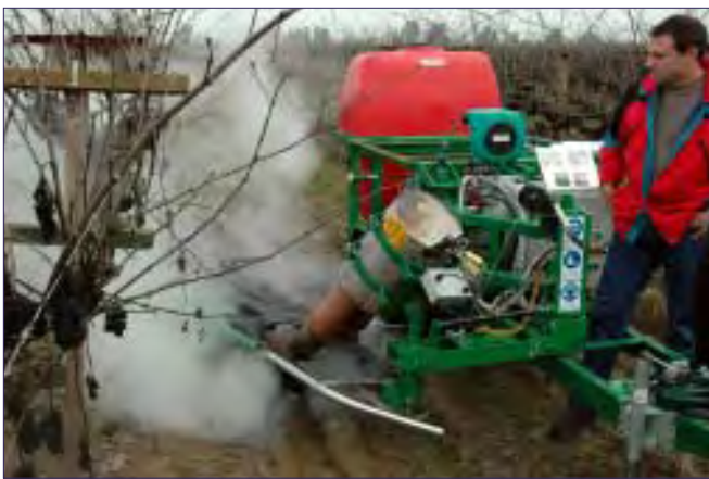
A weed steamer eradicates weeds without pesticides, tillage or damage to irrigation lines.
