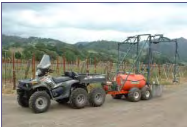
A six-wheel ATV that pulls a double-boom sprayer was one of the winery's custom solutions for treating more acreage more quickly without compressing down the soil or cover crops.
