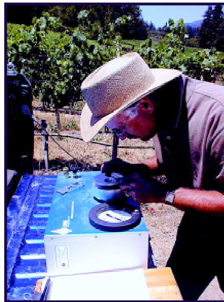
Randle Johnson of Hess Collection Winery takes a water status reading with pressure chamber equipment.
